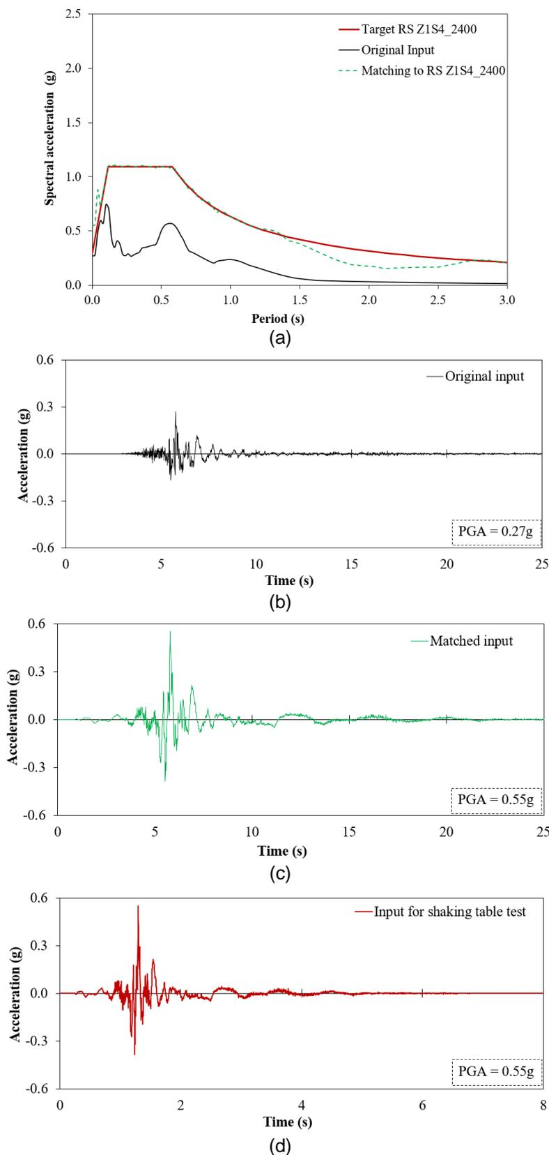
Fig. 2. Input ground motions: (a) response spectrum; (b) original acceleration time history; (c) matched acceleration time history; (d) acceleration time history for shaking table test
