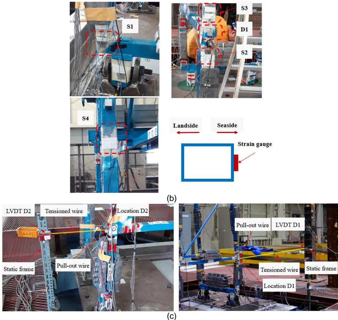
Fig. 1. (a) The 1/20 scale container crane; (b) Installing strain gauge; (c) Installing LVDT
