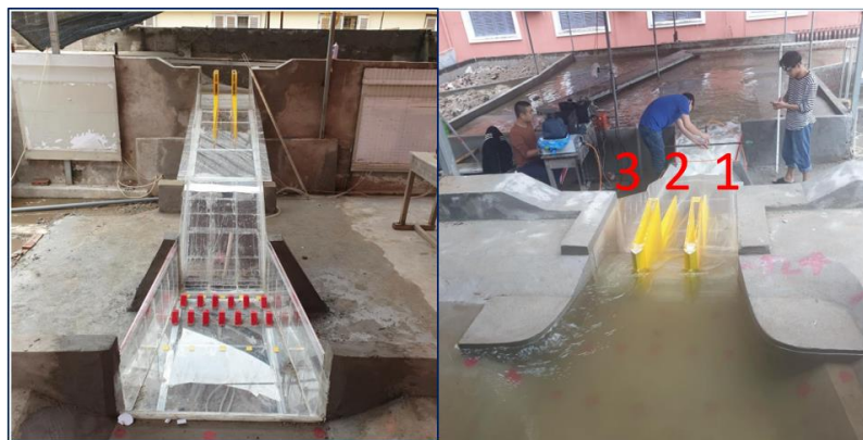
Figure 2. Experimental model of the Ta Hoet spillway and location of gates (from [14])
